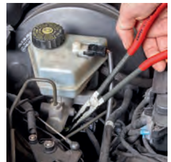
Wave-shaped gripping profile: transverse profile for gripping, holding and guiding
