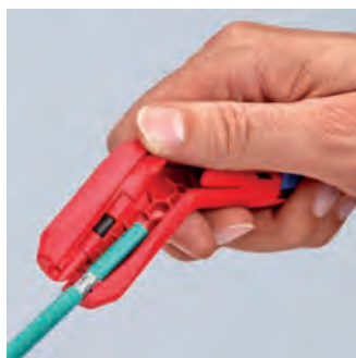
Stripping of a data cable
