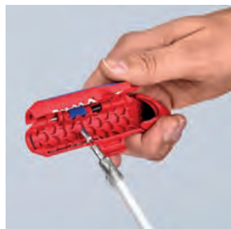
Stripping of a coax cable
